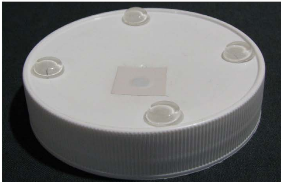
Figure 9 — Bottom of measurement tray with adhesive rubber feet.
