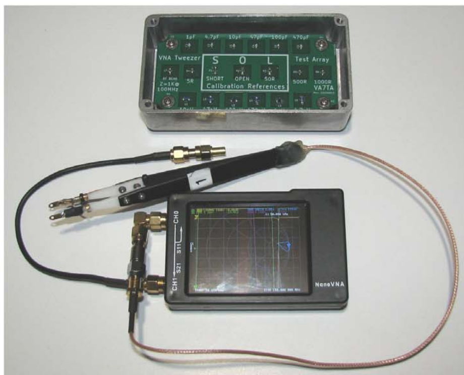
Figure 1 — NanoVNA tweezers connected via 6 dB attenuator.
