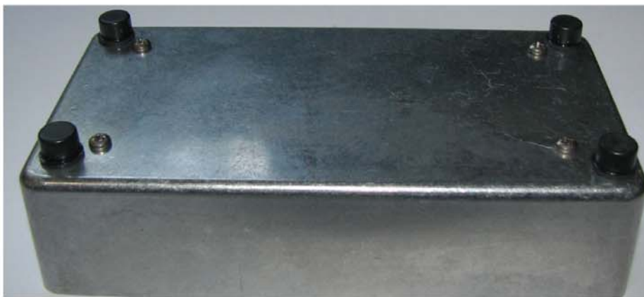
Figure 13 — Rubber feet on bottom of reference box.
