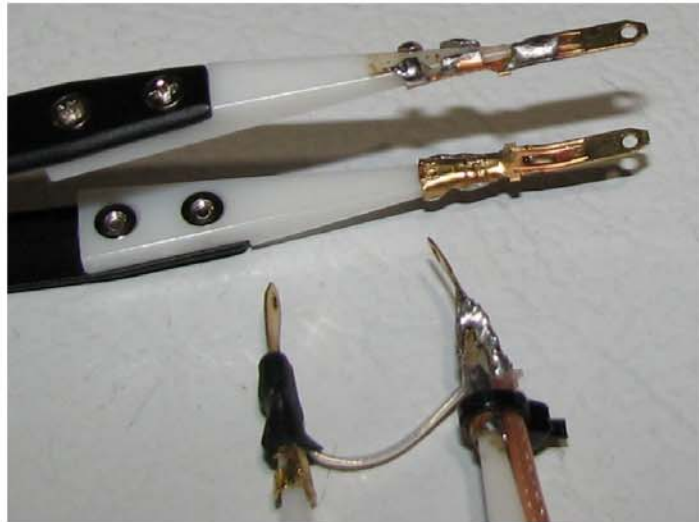
Figure 5 — Spade lug contacts installed and aligned.
